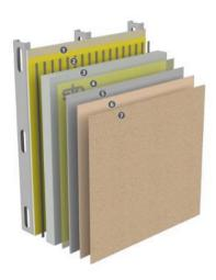
The example to the left highlights the EFIS system with the layers involved.
